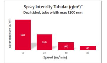
\*The exact coverage on fabric is depending on the fabric characteristics. Chemistry to be formulated for spray application with maximum viscosity at  $8mPa \cdot s$ .
