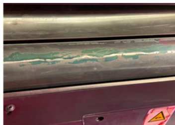
Polyester Typical condition when polyester is removed from the cylinder
